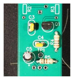
\_\_\_\_ **1.1kΩ Resistor R3** Install R3.
