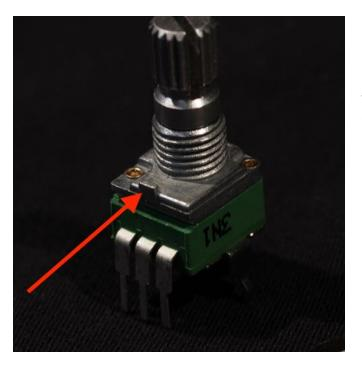
Install the 9mm  $10k\Omega$  audio gain pot at R7.
