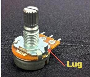
The included potentiometers feature an anti-rotation lug. You'll need to remove the anti-rotation lug. This is easy to do with a small pair of pliers. Just hold the potentiometer firmly in one hand, grasp
