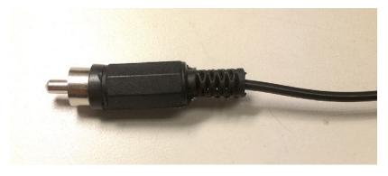
Slide the plug cover back over the plug, and carefully thread it back on. If you like, you can tie a loop knot in the other end of the antenna to make it convenient to hang the end of the antenna on something.
