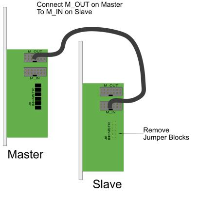
Note that both modules still need to be connected to the Eurorack power bus with their own cable.
